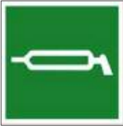
ATTENTION: Lubrication point
