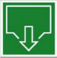
ATTENTION: Drain point.
