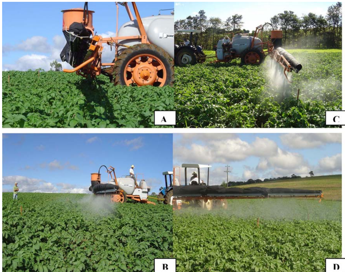
Figure 2 – Spraying sleeve boom angulation against the tractor-sprayer assembly displacement (A and B), and in favor of the displacement (C and D).
