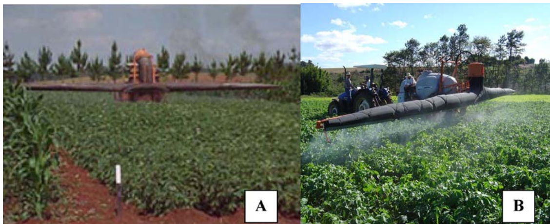
Figure 1 –Sprayers with air assistance near the spraying sleeve boom in the potato cultivation: Falcon Vortex (A) and Advance Vortex (B).
